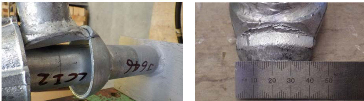
Figure 4: Cup split and tongue fracture
