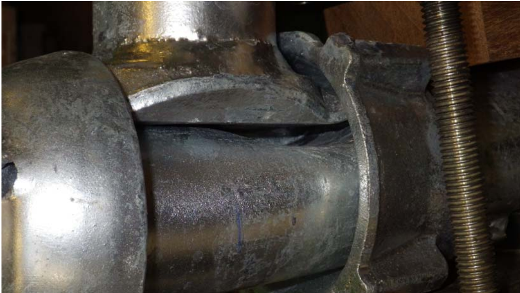
Figure 14: Standard distortion at joint
