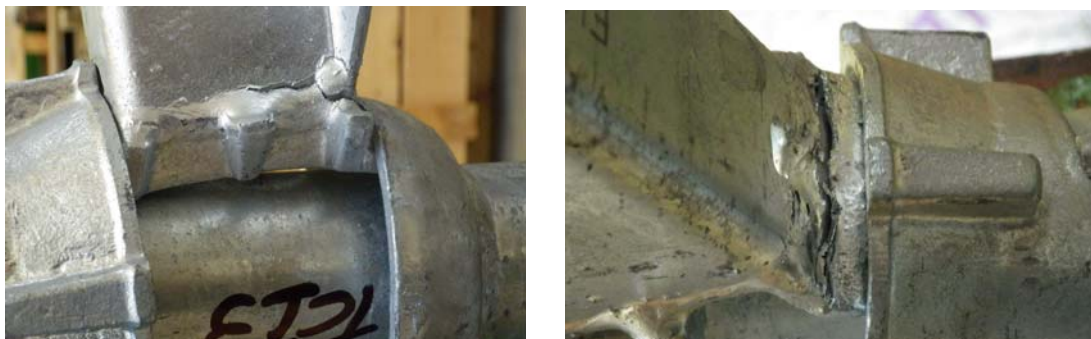
Figure 5: Weld and tongue fracture
