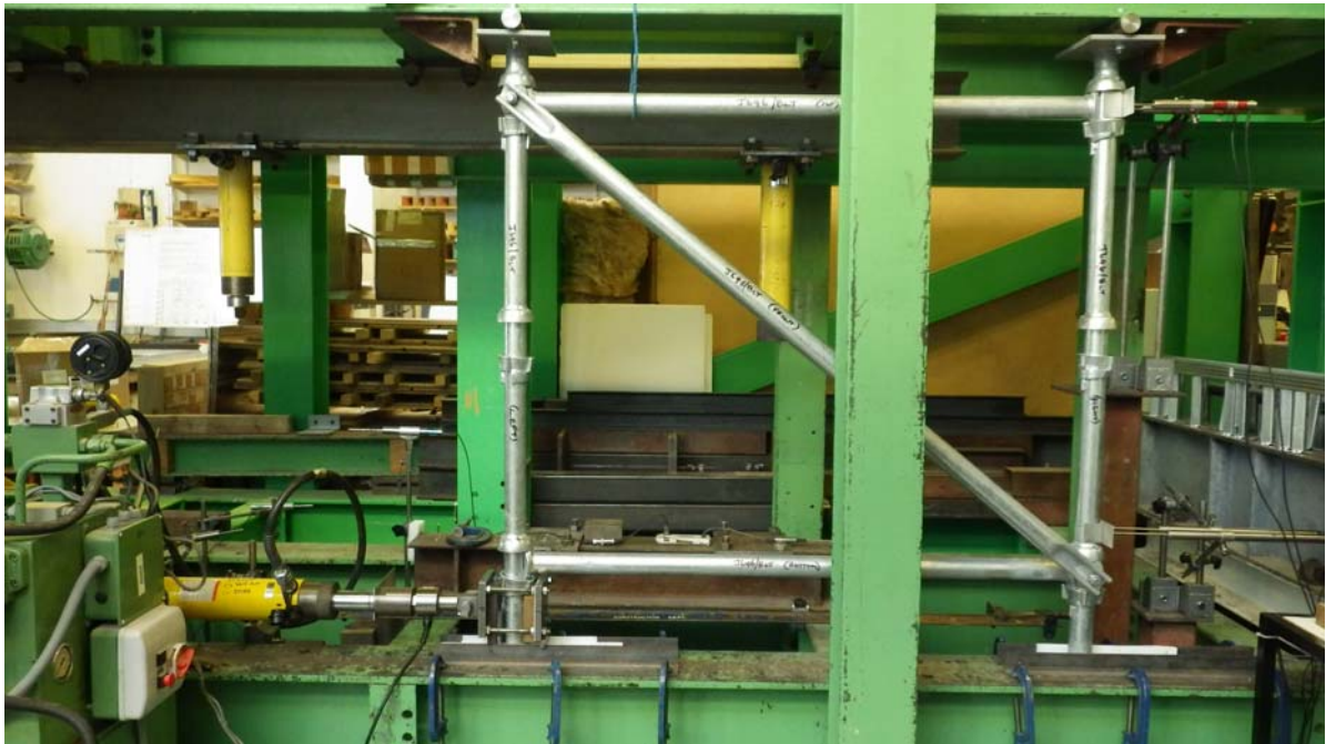
Figure 10: General view of test arrangement (tension)
