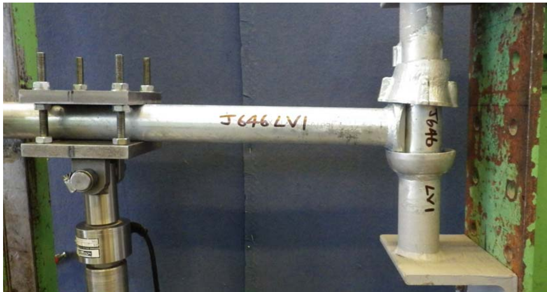
Figure 3: Ledger to standard connection test arrangement (negative rotation)
