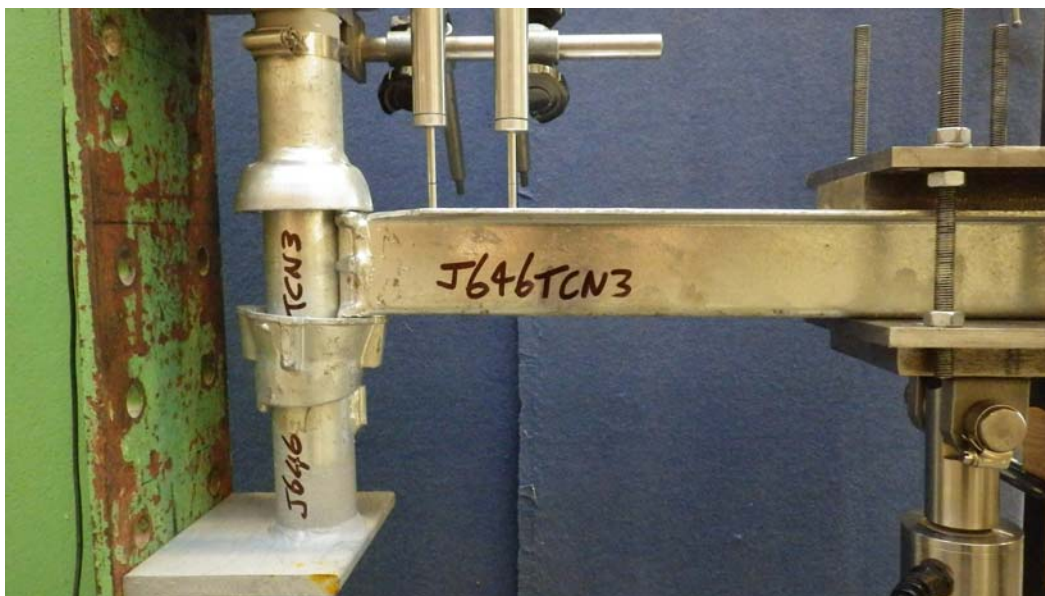
Figure 2: Transom to standard connection test arrangement (positive rotation)
